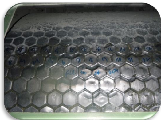
HEXADUR® surface after 53700 hours of operation.
