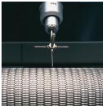
Meßmaschine zur Qualitätssicherung Measuring equipment for quality control
