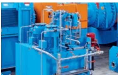
Hydraulic power pack
